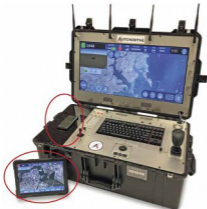
New GCS software is enabling control and monitoring of large numbers of unmanned systems from multiple different devices simultaneously (Courtesy of Autonomy)
